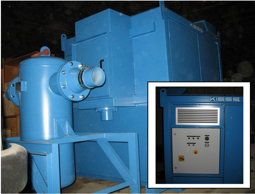
Fig. 19. General view of Vacuum Extractor aggregate type DV 3001 D KI ESS including cyclone pollutants separator
