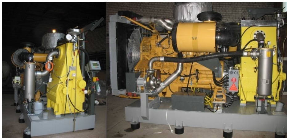
Fig. 18. General view of high efficient ( Q_{\max}=155 dm 3 /min) diesel hydromonitor equipped with high-pressure ( p_{\max}=150 MPa) pump type HDP 483
