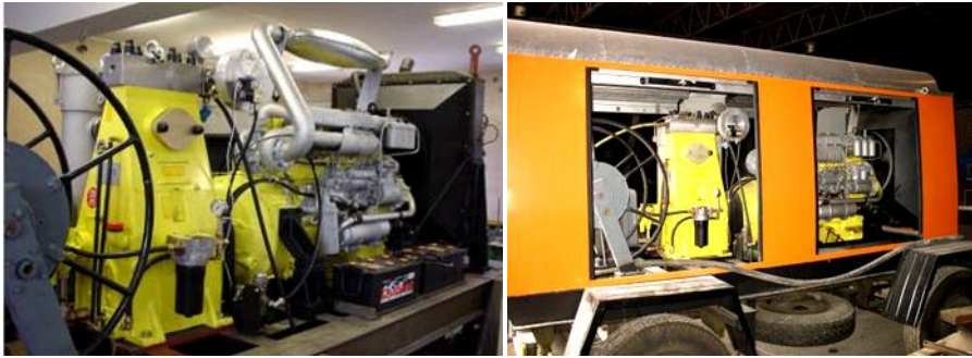
Fig. 12. General view of mobile high-pressure hydromonitor including high-pressure pump type HDP 164 ( p_{\max}=300 MPa, Q_{\max}=30 dm 3 /min)
