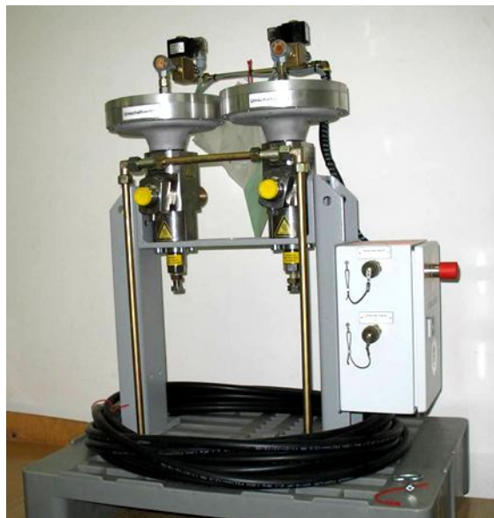
Fig. 8. Example of high-pressure multi stand safety valve type ECMTV 3000
