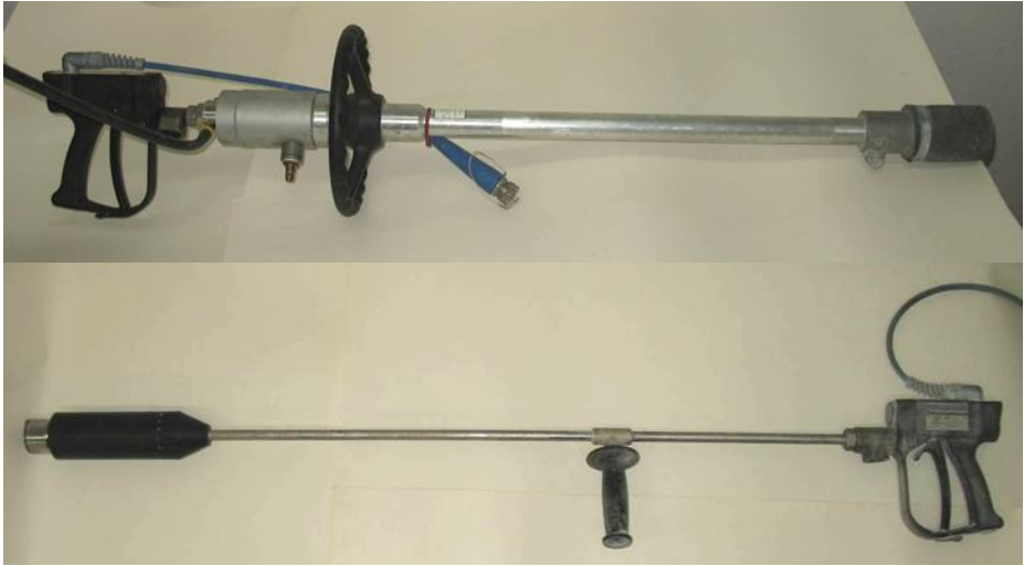
Fig. 4. Examples of high-pressure rotating guns type SP 3000 PR2 (above) and SP 3000E (below)
