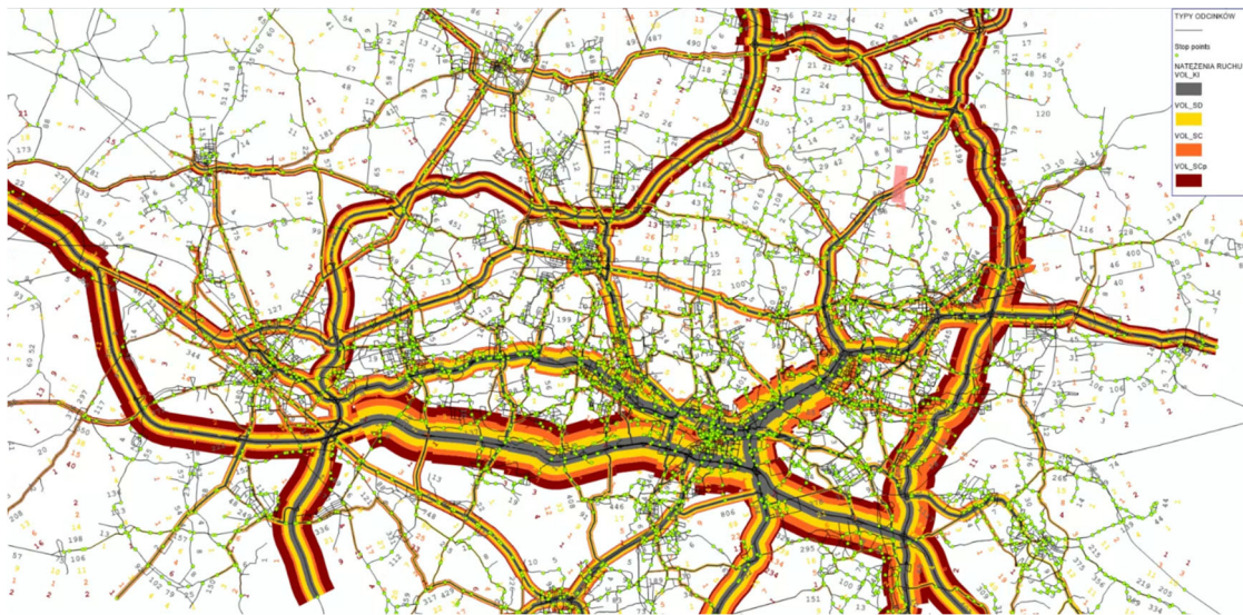
Fig. 2. Map of the traffic volume on the links in the GZM metropolis
