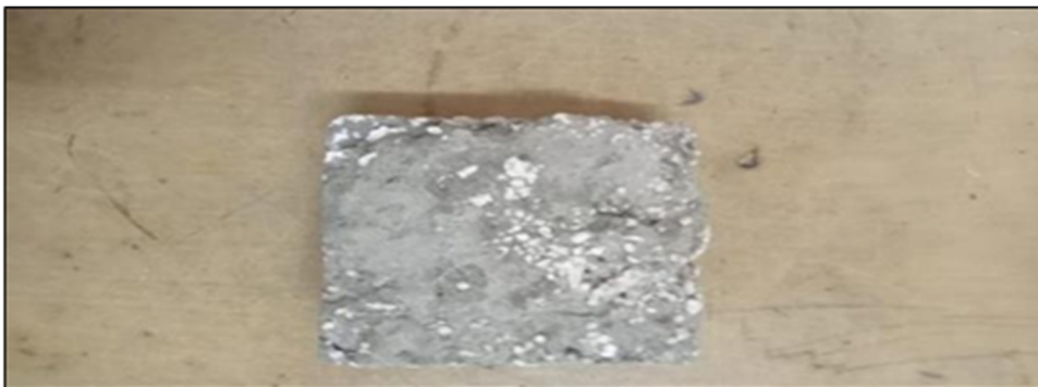
Fig. 13. EPS specimen for testing
