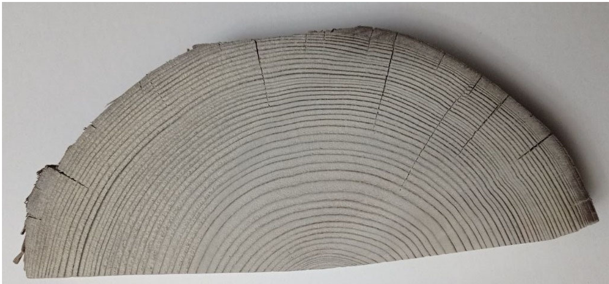
Fig. 3. Cracks of the peripheral part of the studied log
