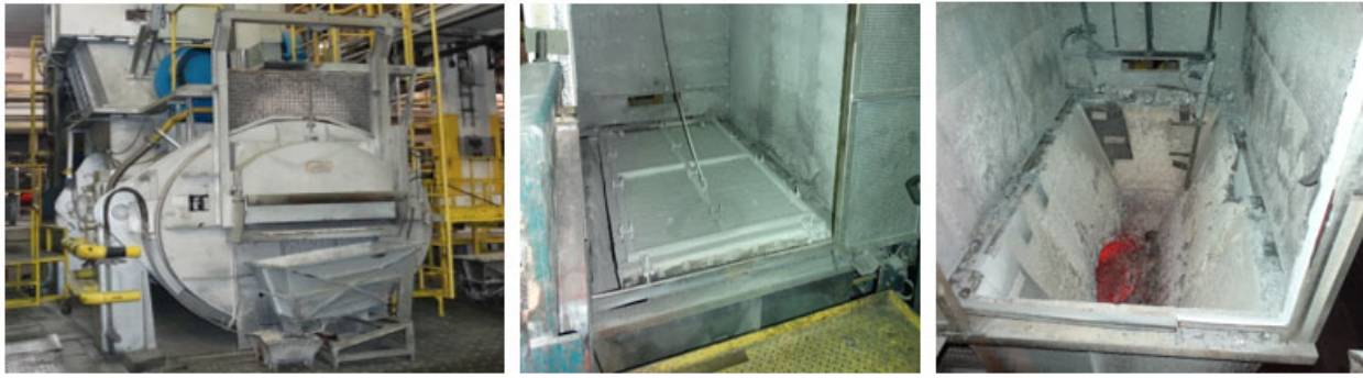
Fig. 3. Melting furnace with an example of an inner lining of the melting space
