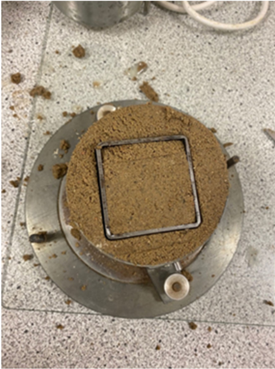
Fig. 4. The scheme of composite Material collection using a knife from the lower cylinder of the Proctor Apparatus
