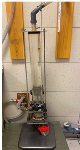
Fig. 3. Soil permeability testing apparatus
