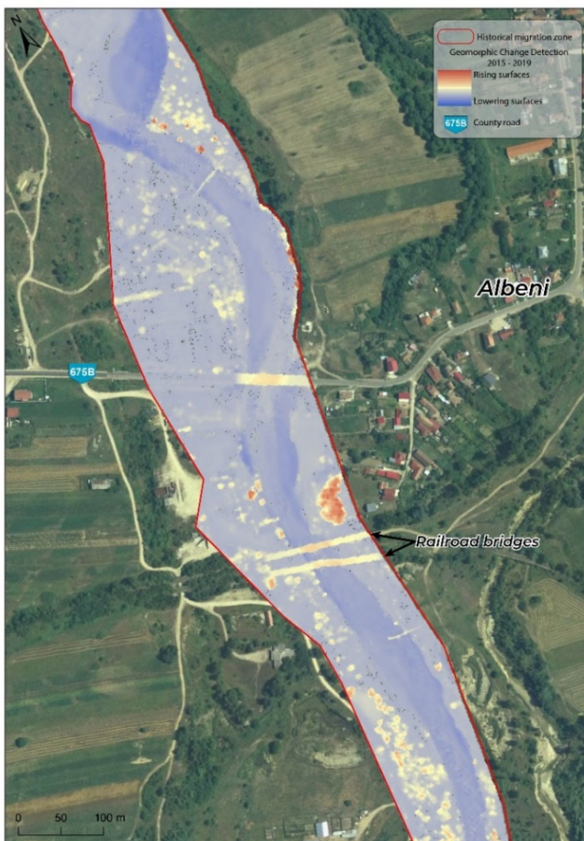
Fig. 6. GCD results at Albeni town bridges
