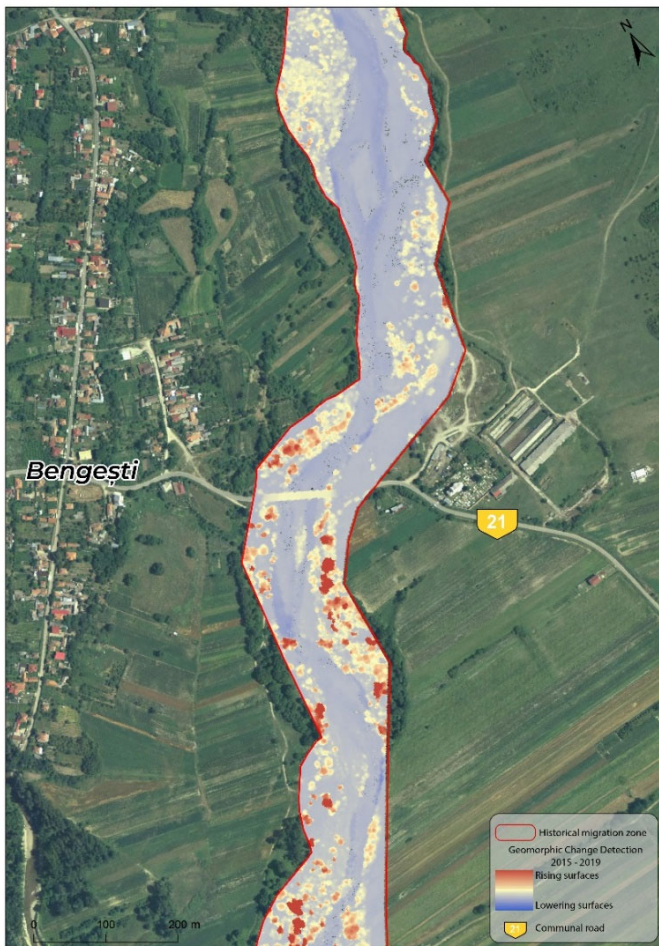
Fig. 4. GCD results at Communal Road 21 bridge
