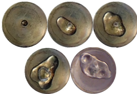
Fig. 5. Instabilities during evaporation of the water droplet from the heating base
