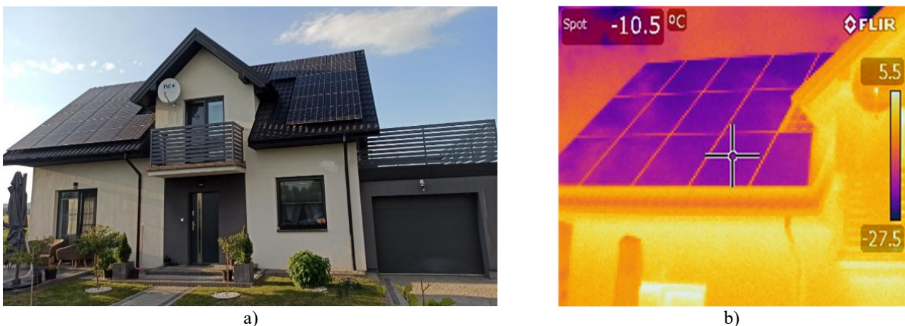
Fig. 1. The front facade of the single-family house: a) digital photo, b) infrared image
