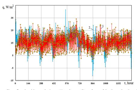
Fig. 8. Distribution of heat flux densities on the inner (1) and outer (2) surfaces of the three-chamber glass unit
