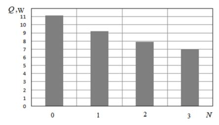
Fig. 5. Dependence of the integral heat flux transferred through a three-chamber glass unit on the number of lowemission coatings
