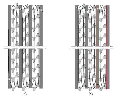
**Fig. 1.** Temperature field (°C) and directions of velocity of the gas medium in the vertical section of three-chamber double-glazed windows: a) without coatings, b) with three coatings
