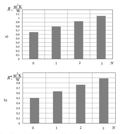
**Fig. 6.** Dependence of the heat transfer resistance of a three-chamber glass unit on the number of low-emission coatings: a) total resistance, b) own resistance
