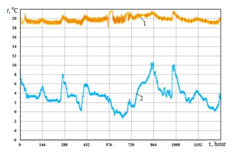
Fig. 7. Temperature distribution on the inner (1) and outer (2) surfaces of three-chamber glass unit
