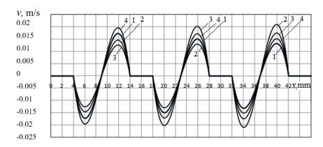
**Fig. 2.** Comparison of vertical velocity distributions in air layers along the thickness of a three-chamber glass unit: 1) without coatings, 2) one coating, 3) two coatings, 4) three coatings
