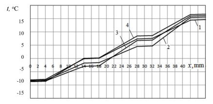
**Fig. 3.** Comparison of temperature distributions across the thickness of a three-chamber double-glazed unit: 1) without coatings, 2) one coating, 3) two coatings, 4) three coatings
