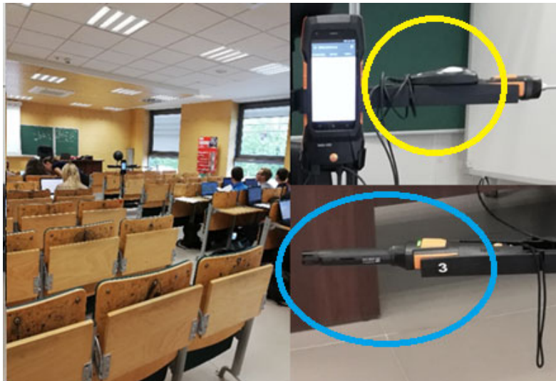
Photo 2. Testo 400 microclimate meter with probes: light intensity (yellow circle) and air temperature and humidity (blue circle)
