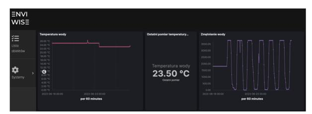
Fig. 4. Test charts of the central application dashboard - data from the temperature and water turbidity sensor
