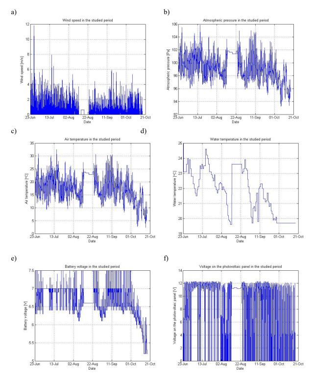
Fig. 8. Collected data by the buoy in the period from June 23 to October 18
