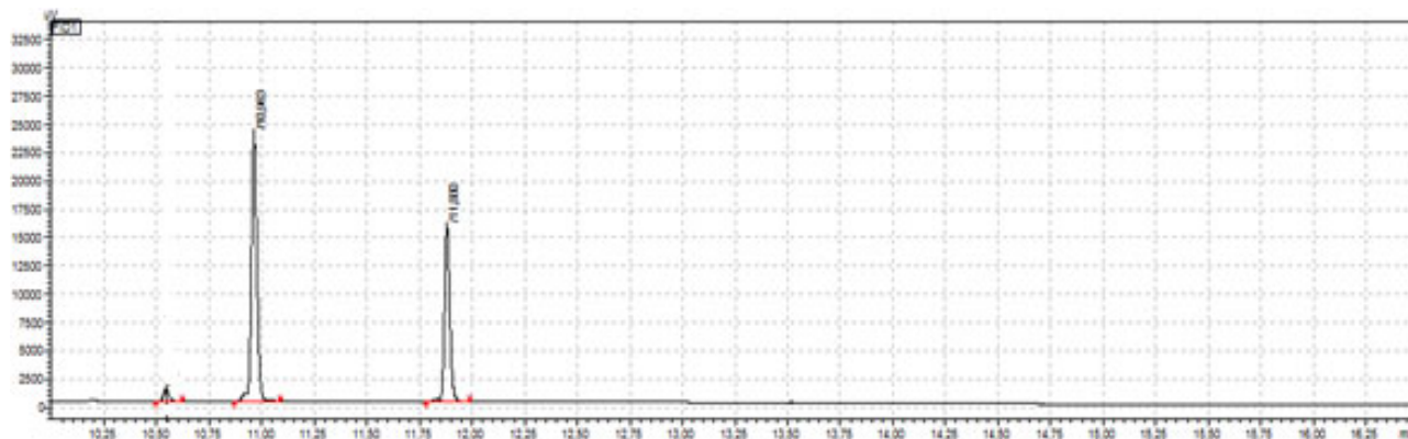
Fig. 4. Chromatogram obtained with the extraction of DBP from aqueous solutions of phthalates (RT = 10.962 – retention time for BB, RT = 11.879 – retention time for DBP)
