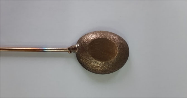
Fig. 4. Crucible for casting the anode
