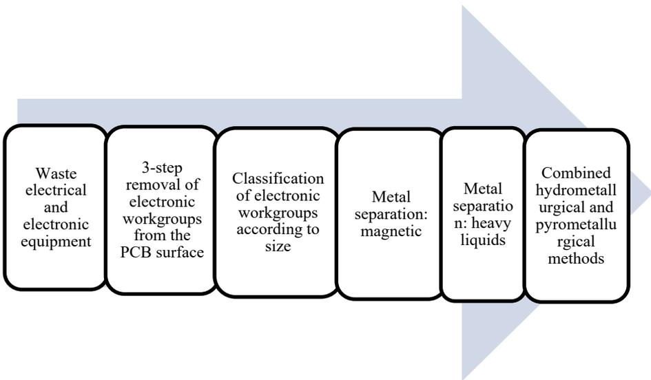
**Fig. 5.** A sample scheme of waste material flow which enterprises should use in their plants
