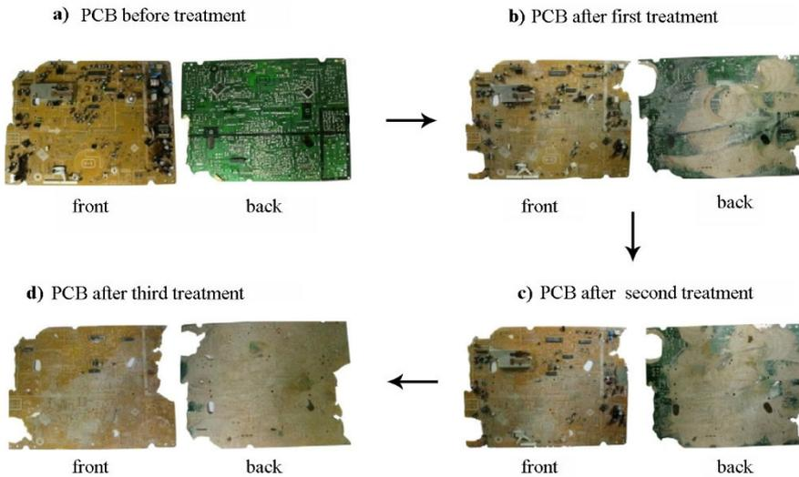
**Fig. 3.** PCB processing using three combined methods
