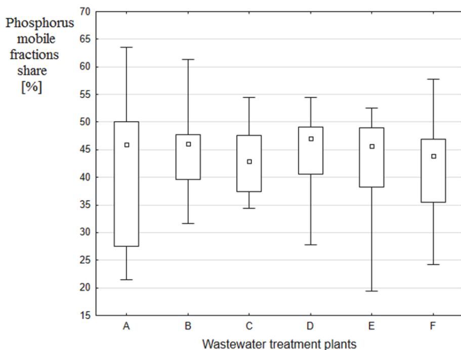
**Fig. 3.** Shares of phosphorus mobile fractions in activated sludge collected at A, B, C, D, E and F treatment plants
