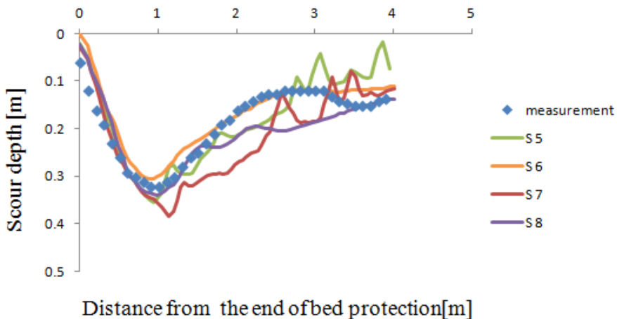
Fig. 5. Longitudinal profiles of local scour holes simulated by SSIIM code on the basis of [14] research, experiment H, after 8 h of erosion
