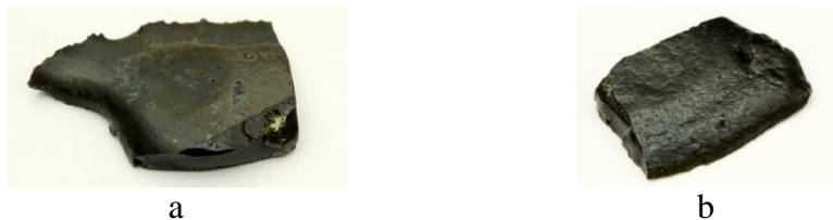
Fig. 2. Vitrificates obtained during plasma modification: (a) ash after sewage sludge combustion; (b) ash after combustion of sewage sludge with the 20% addition of dolomite post-floatation waste
