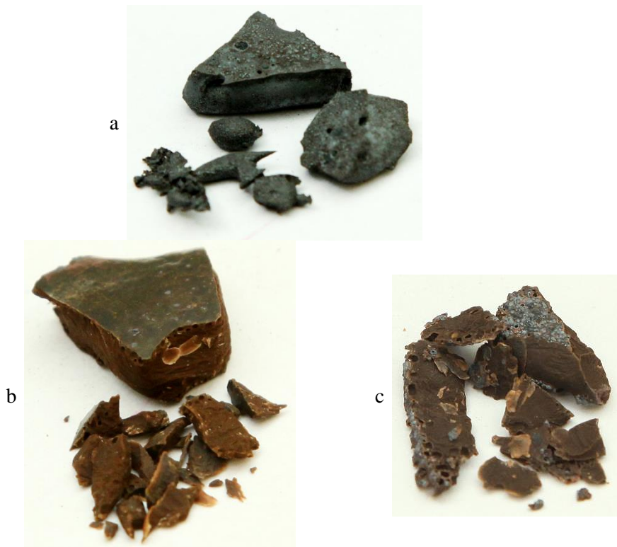
Fig. 5. Devitrification products for the vitrificates obtained from: (a) ash after sewage sludge combustion (crystallization temperature: 1150°C); (b) ash after combustion of sewage sludge with the addition of dolomite post-flotation waste (crystallization temperature: 871°C); (c) ash after combustion of sewage sludge with the addition of dolomite post-flotation waste (crystallization temperature: 986°C)
