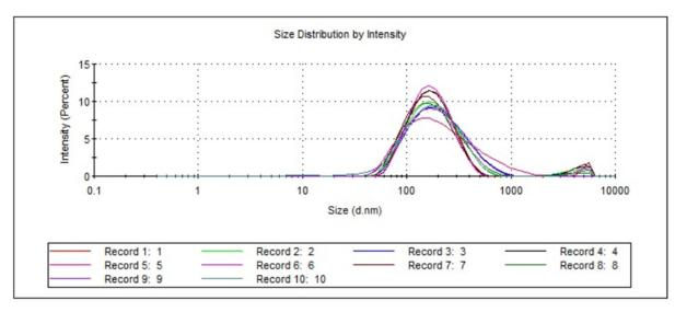
Fig. 2. Distribution of the peaks for individual samples containing PE
