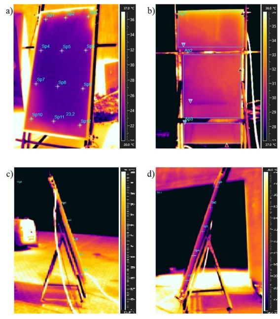
Fig. 7. Thermographic measurements of the collector made for a medium flow rate of  $80 \, [kg/h]$  and a working medium temperature of  $40 \, [^{\circ}C]$ . a) front surface, b) rear surface, c) and d) side surfaces of the collector
