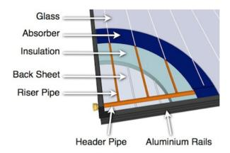
Fig. 3. Construction of a flat plate solar collector
