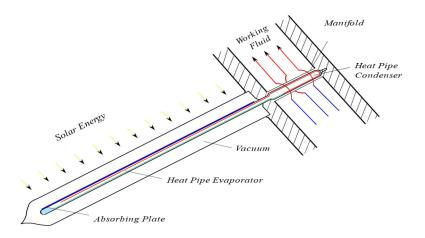
Fig. 2. The principle of vacuum tubes
