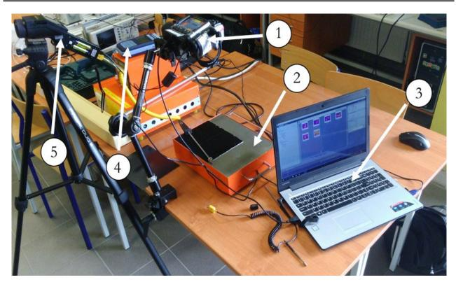
**Fig. 4.** Temperature distribution measuring stand; 1 – Thermovision camera, 2 – Heat plate, 3 – computer, 4 – hygrometer, 5 – pyrometer
