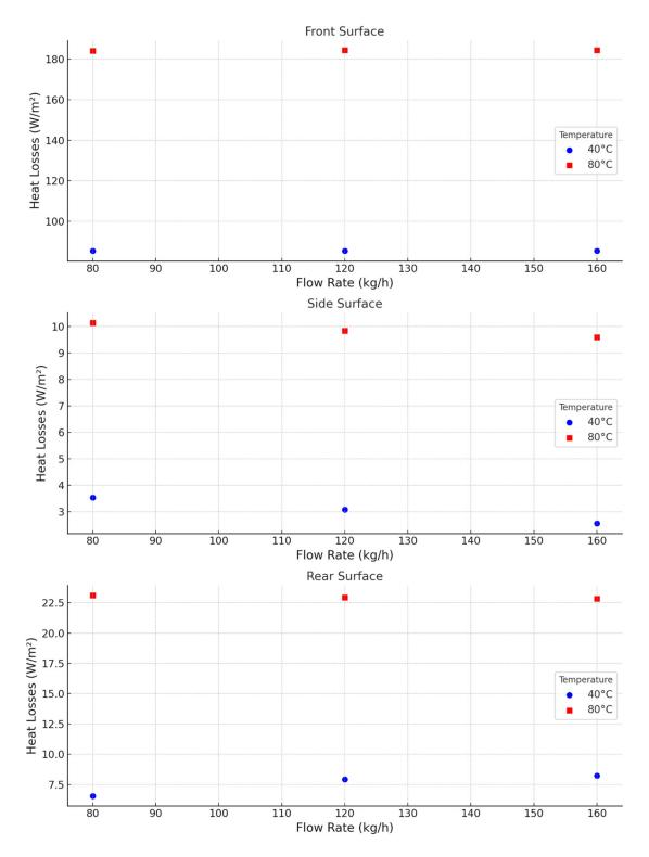
Fig. 9. Heat loss characteristics at different temperatures and surfaces
