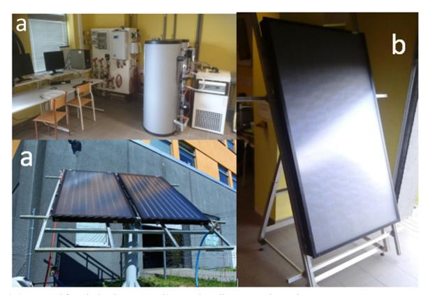
Fig. 6. a) Test stand for solar heating systems; b) new solar collector mounting station
