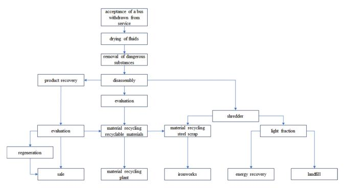
Fig. 2. General diagram of the end-of-life bus recycling process, based on (Tomczyk 2012)
