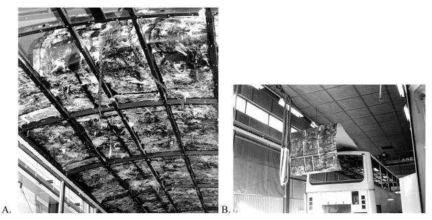
Fig. 8. A – Removal of the entire wall and ceiling insulation; B – Removal of the roof using a crane or gantry
