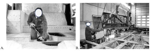
Fig. 12. A-Removal of floor slabs; B-Removal of the body sides
