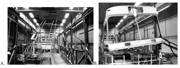
Fig. 10. Removal of the roof; B – Removal of the front by cutting
