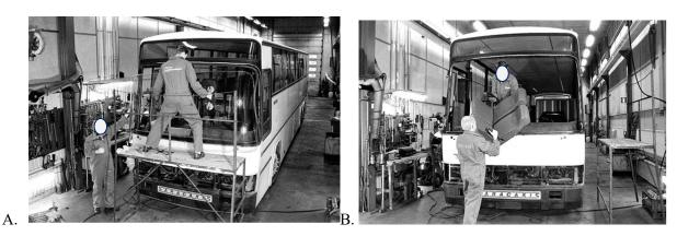
Fig. 4. A – Windshield removal; B – Seats removal
