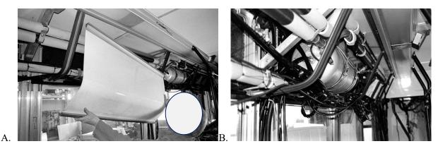
Fig. 6. A – Removal of shelf nets and flaps; B – Removal of door mechanism, air conditioning fan, air tank and electrical wires
