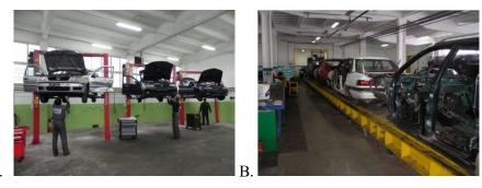
Fig. 3. A - lift used in cell-based dismantling; B - dismantling of components in the dismantling line
