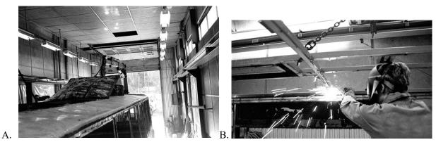
Fig. 9. A - Removal of the roof using a crane or overhead crane; B - Removal of bumpers, all flaps and roof framing
