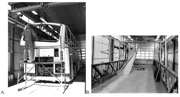
Fig. 11. A - Removal of the rear of the bus; B - Removal of the floor mat
