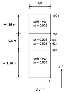
Fig. 2. Calculation area of a shallow horizontal soil heat exchanger
