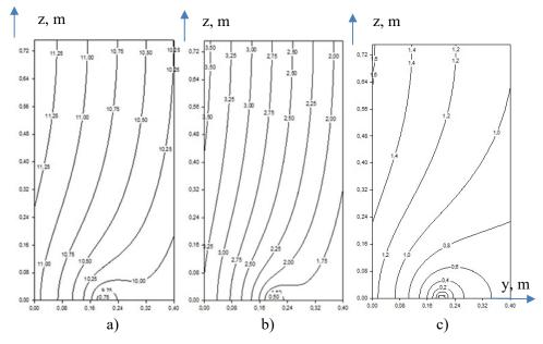
**Fig. 5.** Distribution of temperatures in the soil massif during the operation of a shallow horizontal soil heat exchanger at  $L = 1.5 \text{ m}, \Delta T = 0.05^{\circ}\text{C}$ : a) for November 15; b) for January 15; c) for March 15
