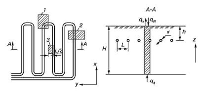
Fig. 1. The design of a shallow horizontal soil heat exchanger
