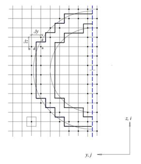
Fig. 3. Calculation area of a shallow horizontal soil heat exchanger pipe
