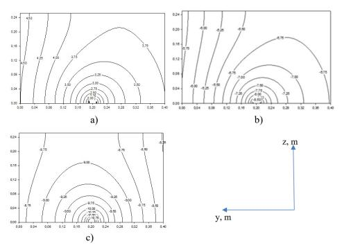
**Fig. 4.** Distribution of the temperatures in the soil massif during the operation of a shallow horizontal soil heat exchanger at L = 0.5 m,  $\Delta T=0.1$ °C: a) for November 15; b) for January 15; c) for March 15
