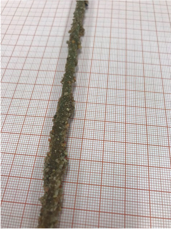
Fig. 2. Sand-resin coating on the PET reinforcing bar
