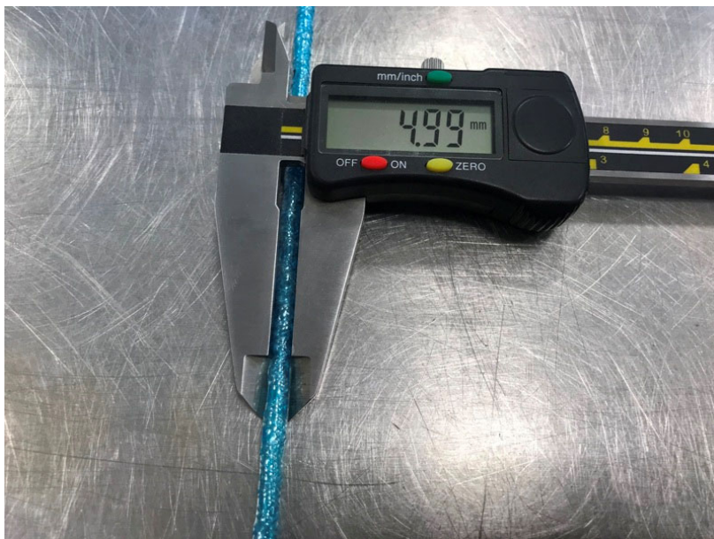
Fig. 3. Determination of a PET bar diameter using an electronic calliper
