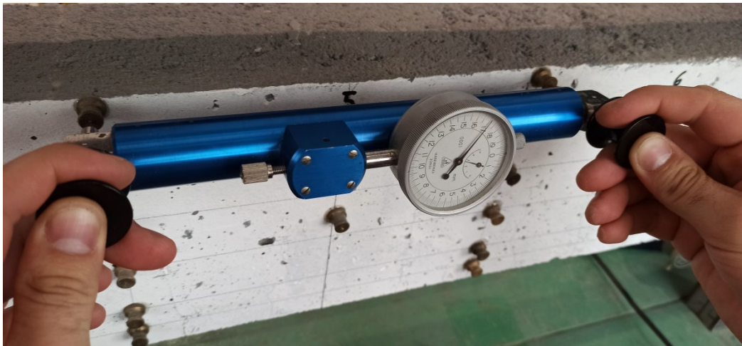
Fig. 6. Measurement of displacements of points on the beam using an extensometer
